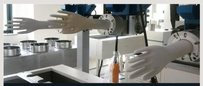
Whole dipping process proceeded by Dipping Instrument of KKPC R&BD CENTER
