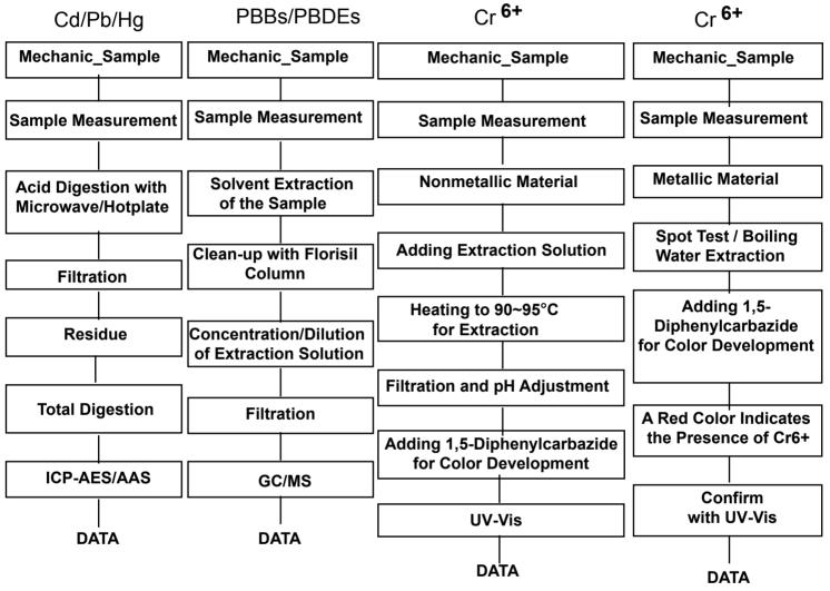
The samples were dissolved totally by pre-conditioning method according to above flow chart for Cd,Pb,Hg. Section Chief : Shapless Park
